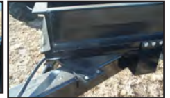
UHMW Wear Plate on Rear Axle
