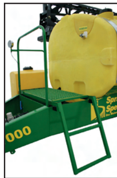
Front end walkway with fold-up steps are Standard on NF Series Sprayers Frames
